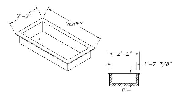
CUT-OUT TO BE 1 3/4" SMALLER THAN OVERALL FLANGE DIMENSIONS
