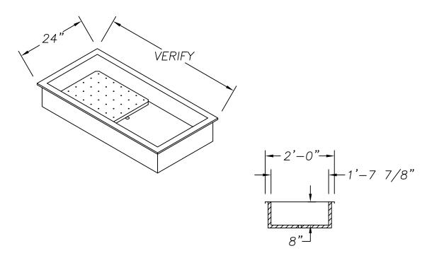
CUT-OUT TO BE 1 3/4" SMALLER THAN OVERALL FLANGE DIMENSIONS
